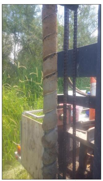
Plate 6: The typical geological profile of boreholes drilled across the site for the Acid Sulfate Soil (ASS) investigation. The profile includes silty sand profiles underlain by clay sand and sandy clay.
